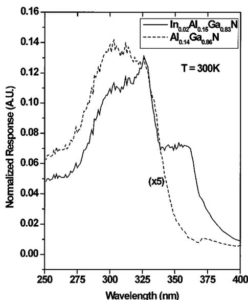
FIG. 3. The response of an  $\text{In}_x\text{Al}_y\text{Ga}_{1-x-y}\text{N}$  quaternary alloy (solid line) and  $\text{Al}_y\text{Ga}_{1-x-y}\text{N}$  alloy (dotted line) with comparable cutoff wavelength. The compositions for these samples are estimated to be  $\text{In}_{0.02}\text{Al}_{0.15}\text{Ga}_{0.83}\text{N}$  and  $\text{Al}_{0.14}\text{Ga}_{0.86}\text{N}$ , respectively.
