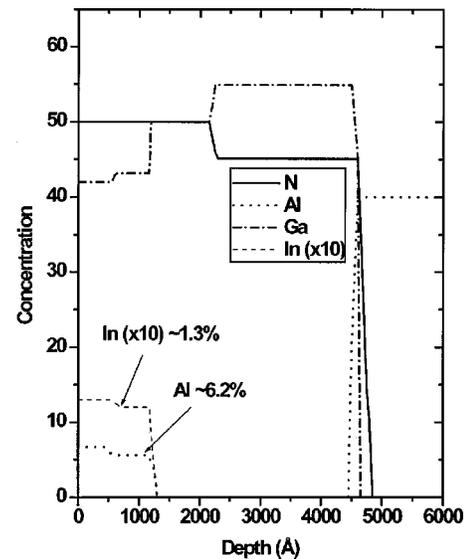
FIG. 1. Rutherford backscattering (RBS) analysis of In<sub>x</sub>Al<sub>y</sub>Ga<sub>1-x-y</sub>N quaternary alloy grown on top of GaN epilayer (No. 706). This sample is found to contain 1.3% indium and 6.2% aluminum (atomic composition). This is close to the composition predicted theoretically for lattice matching to GaN ( $x:y=1:4.7$ ).
