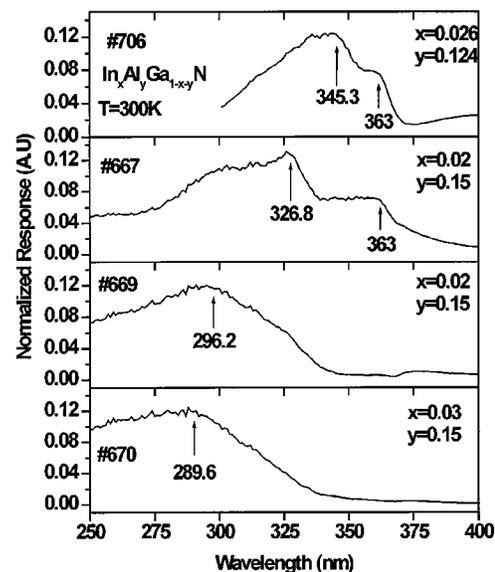
FIG. 2. Normalized photoresponse VS wavelength of incident light of In<sub>x</sub>Al<sub>y</sub>Ga<sub>1-x-y</sub>N quaternary alloys with different In and Al contents. The arrows indicate the cutoff wavelength for the quaternary alloys. The photoresponse from the underlying GaN epilayer in the two samples Nos. 706 and 667 is seen in the steps at 363 nm.
